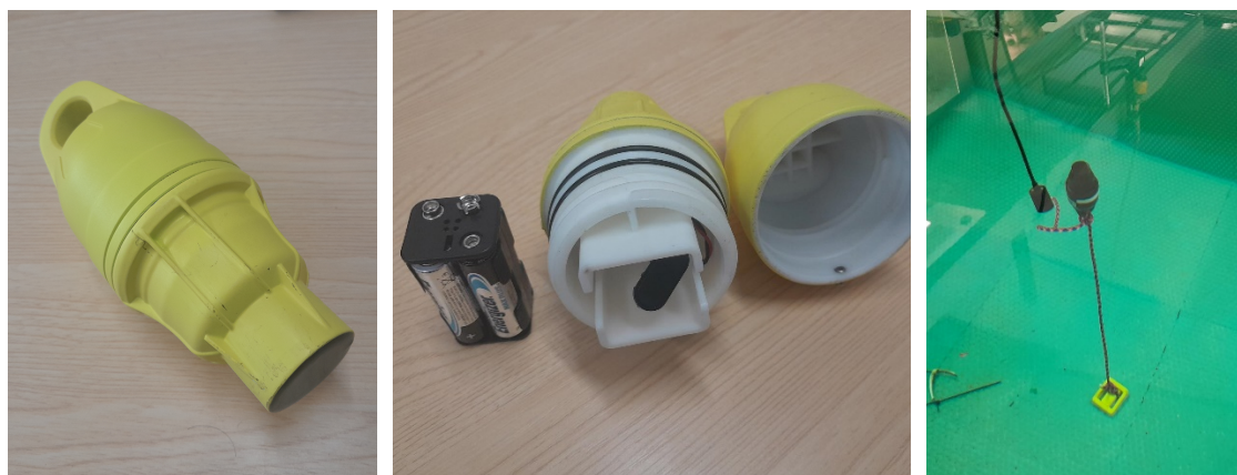
Figure 6. Pre-production NetTag housing, battery enclosure and tank testing
